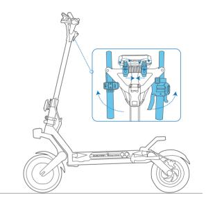
① Loosen the QR lever, pull the locking slide inward and raise the handlebar, then close the QR lever and tighten the set screw.
