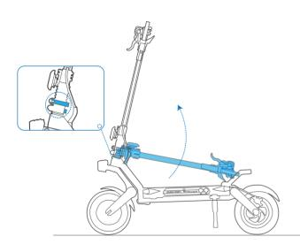
① Release the QR lever,raise the locking slide upwards, raise the steering tube, then lower the locking slide downward.
