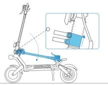
Lay the steering tube down while raising the locking slide.
