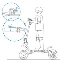
**4.** Slow down by releasing the throttle and squeezing brake levers.
