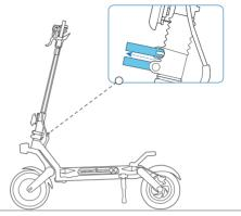
Loosen the QR lever and move the locking slide upward.
