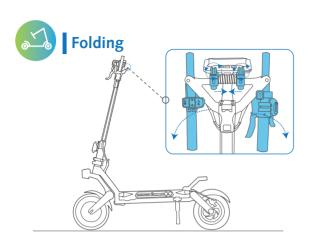
Loosen the QR lever, push the locking slider inward and fold the handlebars down.
