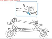
Lock the handlebar hook to the footrest.
